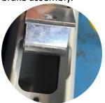
8. Inspect for cracks, Remove debris, and lubricate the O-ring on the caliper pins.
